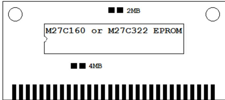
The DxS-GEN24TH-01 has 2 configuration options: **2MB** mode and **4MB** mode. If you're using a 2 MB EPROM (M27C160), solder both 2 MB pads together and if you're using a 4 MB EPROM (M27C322) then solder the 4 MB pads together.
